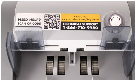
Incorrect Position: Turn rollers until teeth are no longer visible.
